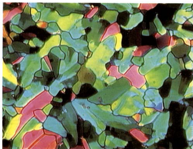
Figure 6. Mosaic texture of the oblique columnar phase of compound DS16 at 173°C (magnification: 100 ×).
