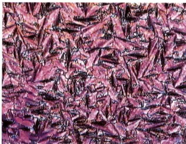
Figure 5. Texture of the oblique columnar phase of compound DS14 at 174°C (magnification: 100 ×, the same sector as in figure 3).
